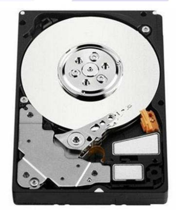
Disk is organized into sectors. The disk arm moves to a spot to read a byte of data
