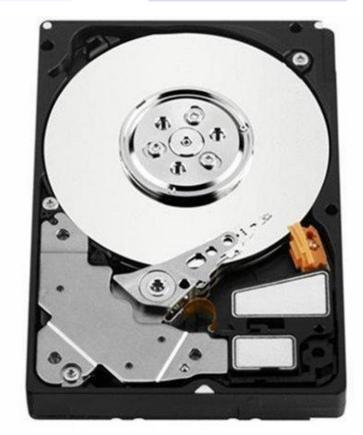
Disk is organize into sectors. The disk arm moves to a spot to read a byte of data
